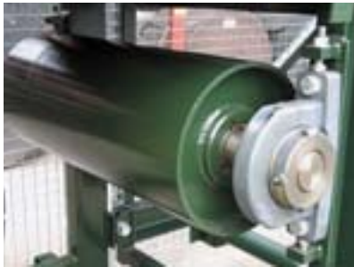
Tension end drum c/w 'Cooper' split bearings.
